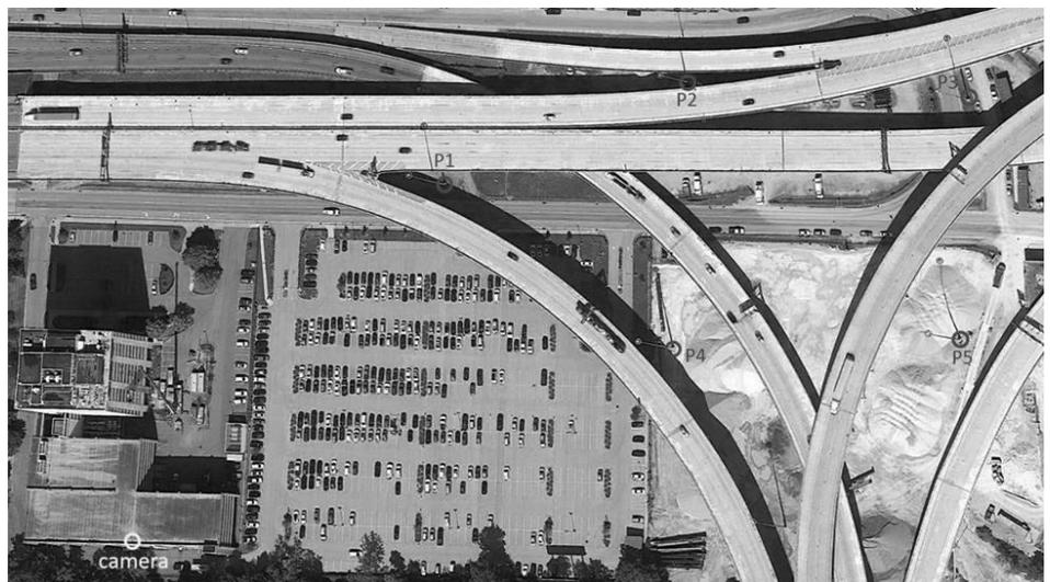
Figure 5. Light poles P1-P5 used for calibration of parking garage camera video.
