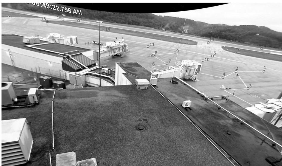
Figure 11. Accident area with superimposed ground track and azimuth direction from the parking garage camera to the airplane.
