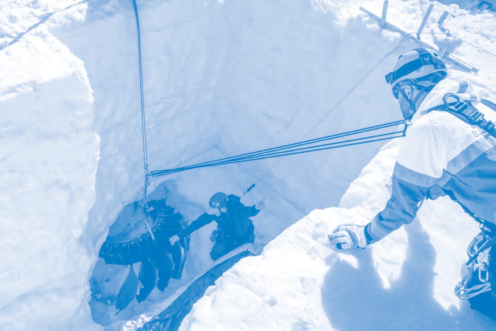
Figure 1. Extraction of fan hub fragment. Source: Austin Lines
