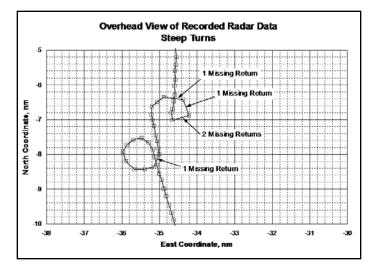
Figure 1. Ground track during steep turns.
