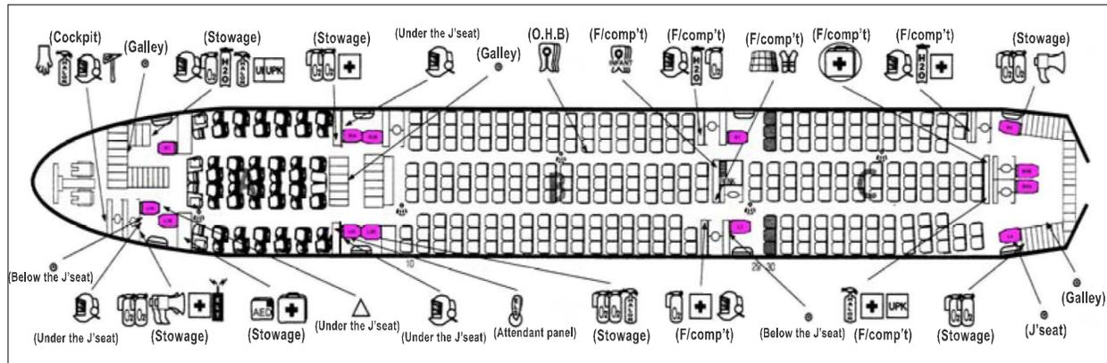
**Figure 7-4. Example of safety and emergency equipment location diagram (Source: NTSB)**
