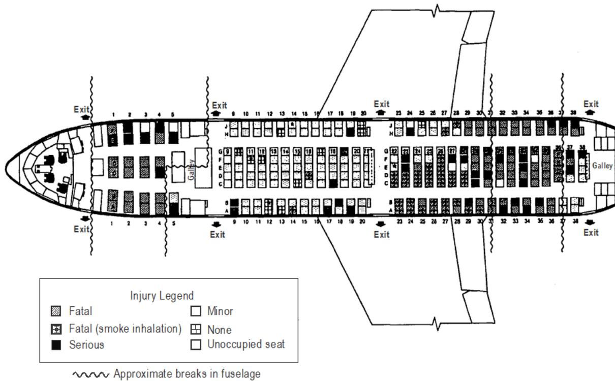
**Figure 7-6. Example of an occupant injury diagram (Source: NTSB)**
