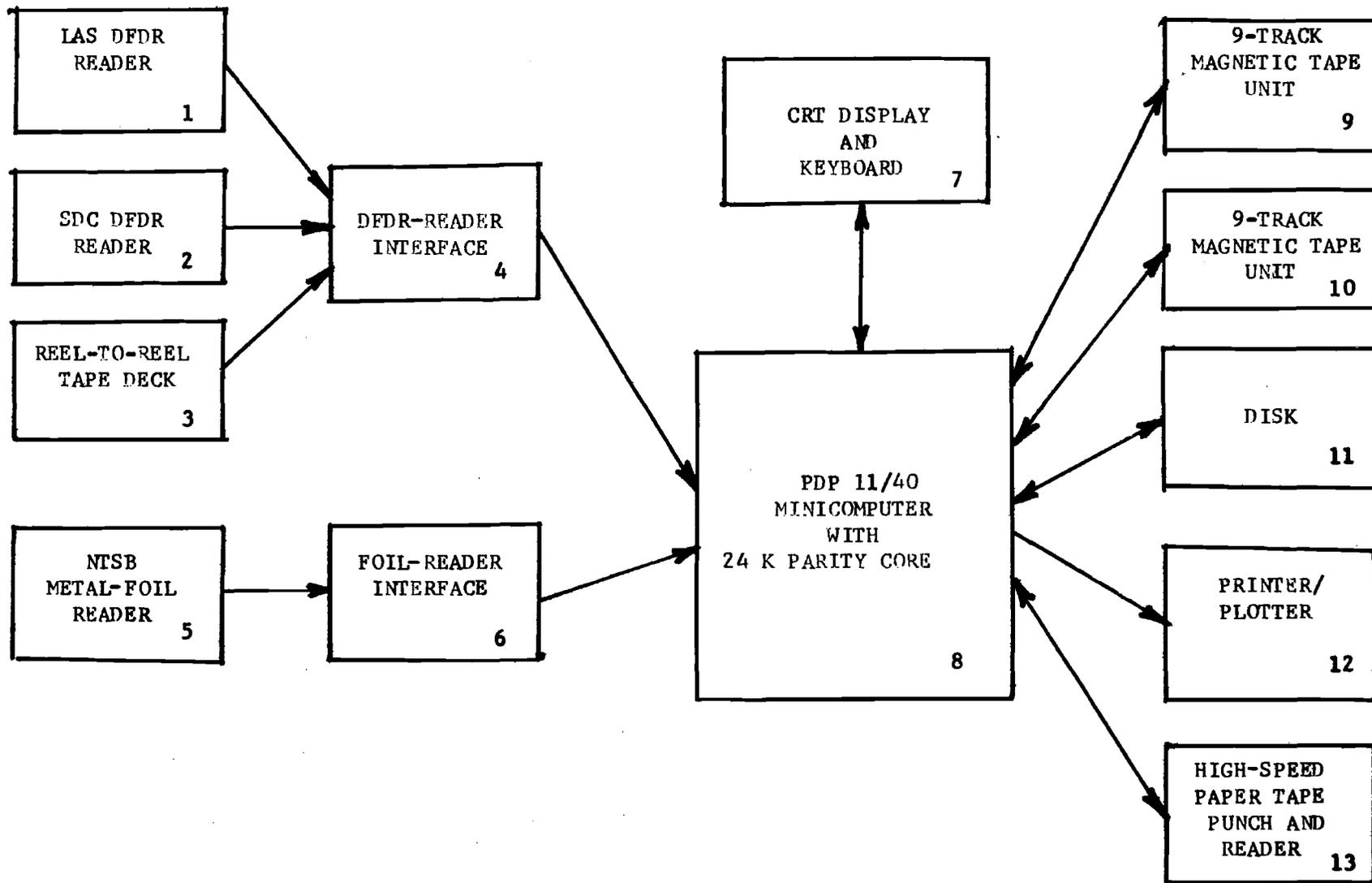
FIGURE 5. National Transportation Safety Board Data Reduction Station.
