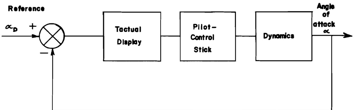
Fig. 1. Control Loop for Angle of Attack
