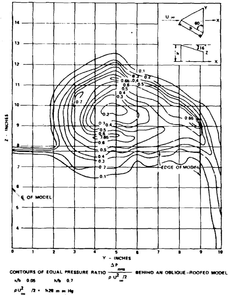
FIGURE 19. STRUCTURE OF LONGITUDINAL BUILDING VORTICES [42].
