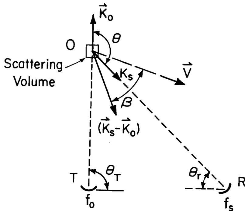
FIGURE 1. Wave Vector Diagram Showing the Component of the Wind Measured by a Doppler Shift
