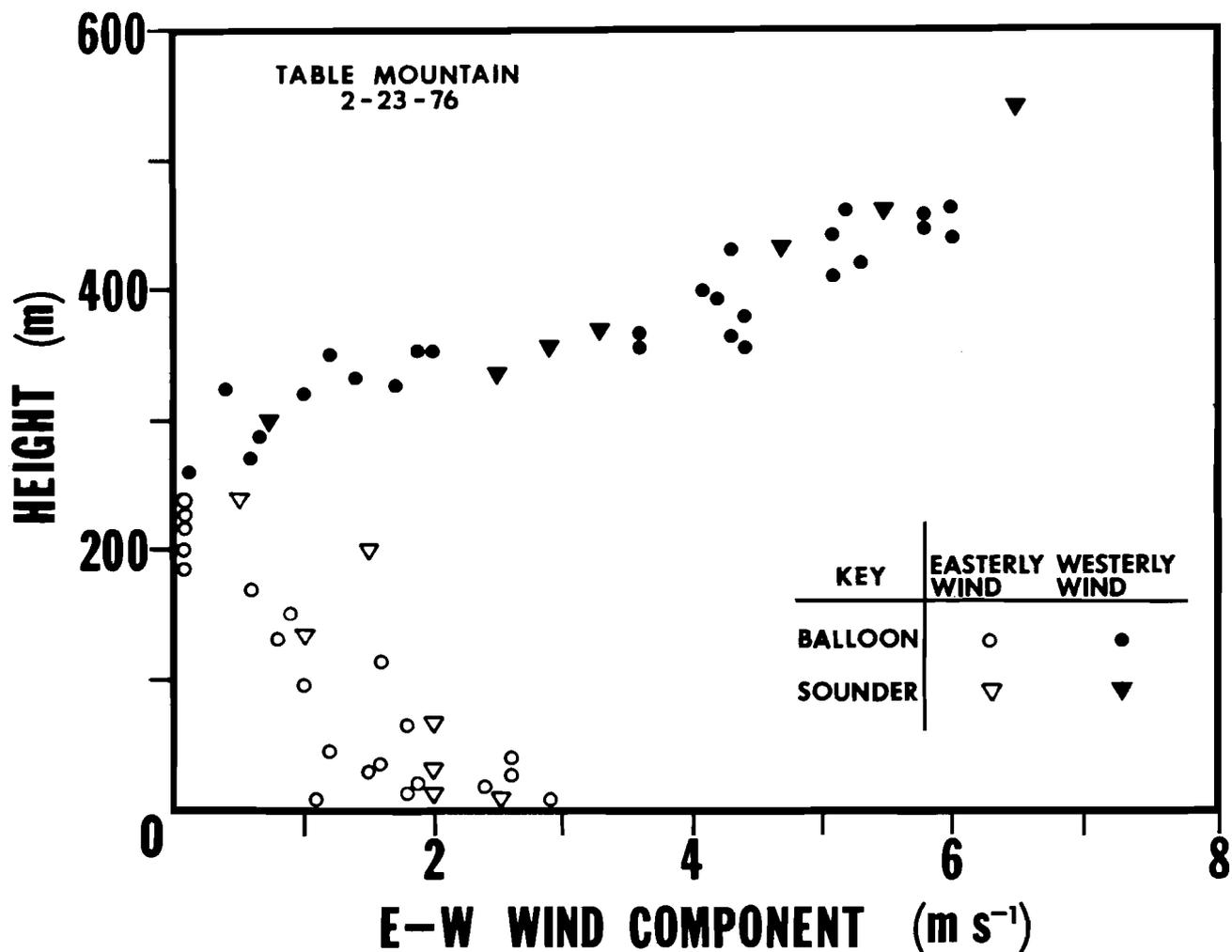
**COMPARISON OF WIND PROFILES MEASURED BY WPL ACOUSTIC ECHO SOUNDER AND BALLOON-BORNE ANEMOMETER**
