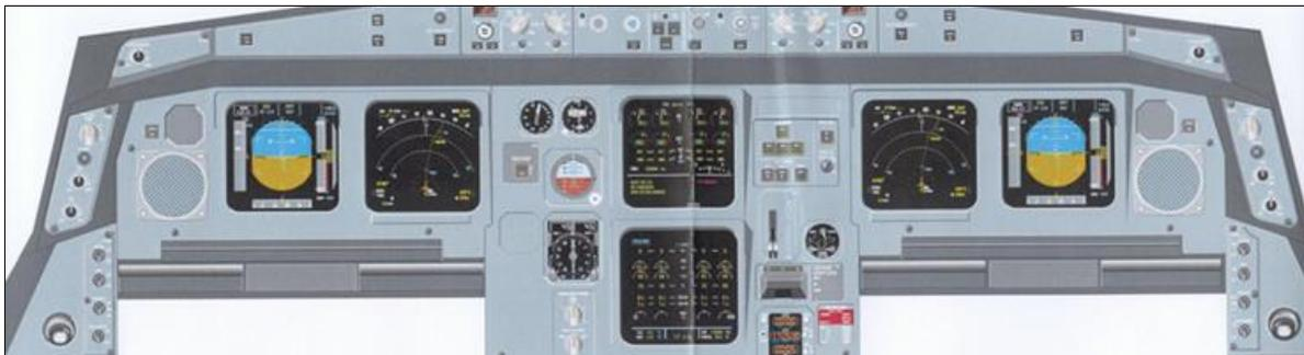
Figure 19. Airbus 320 Flight Deck (Airbus1982).
