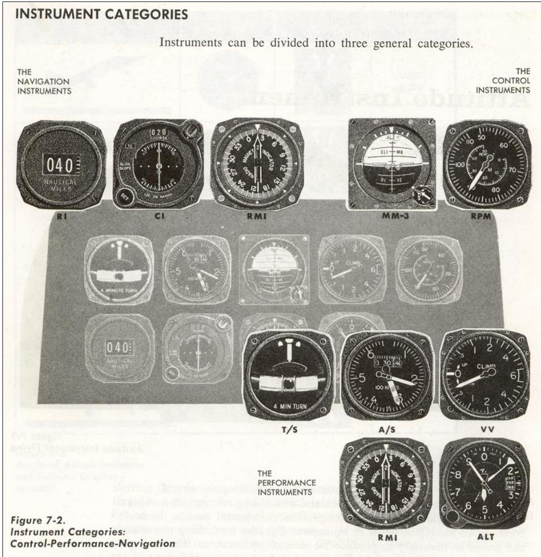
Figure 7-2. Instrument Categories: Control-Performance-Navigation
