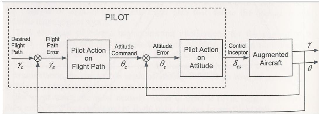
Figure 25. The series pilot model<sup>22</sup>
