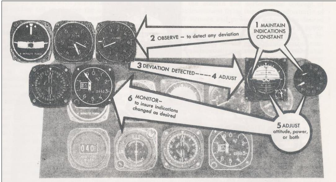
Figure 27. Instrument cross check technique (US Air Force Manual 51-37, 1979).
