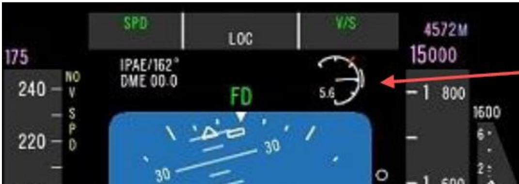
Figure 8. Boeing AOA indicator (Boeing 2013).
