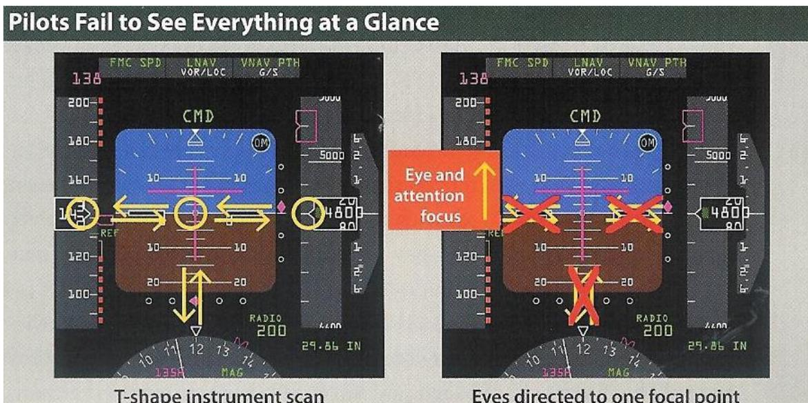
Figure 28. T-shape instrument scan (Boeing 2014).
