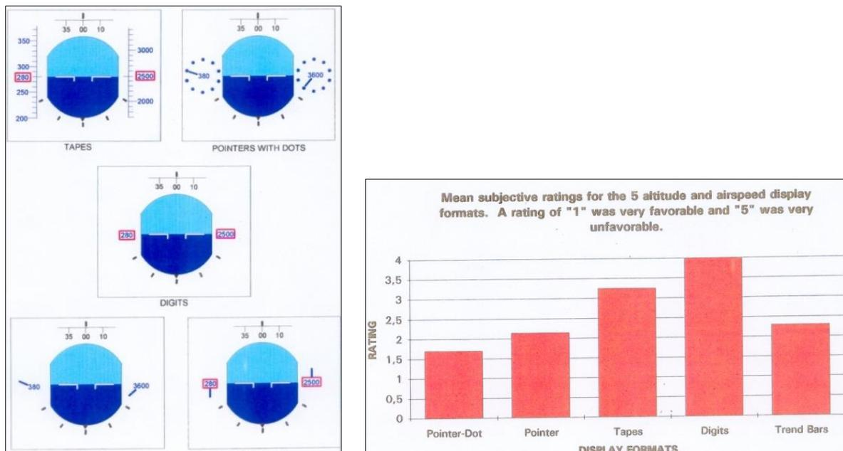
Figure 29. Different types of Airspeed and Altitude displays with Mean Subjective Ratings.<sup>25</sup>
