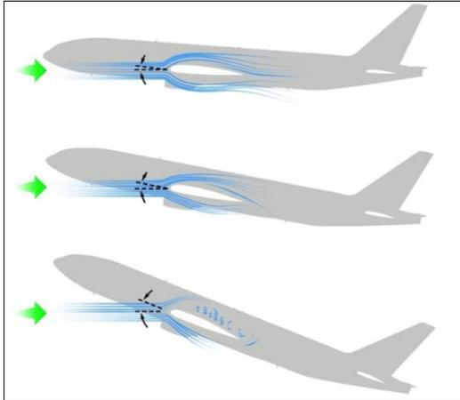
Figure 5. Aerodynamic Stall (D. Carbaugh, Boeing 2010).
